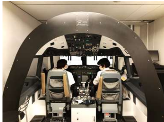
FTD:Flight Training Device (飛行訓練装置)
